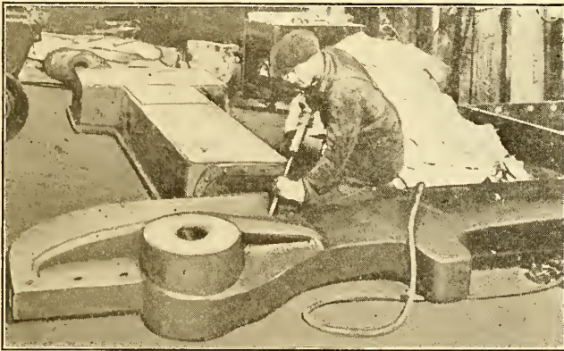
FIG. 129.—An Air Chisel May be Used Either for Grooving or Finishing.
